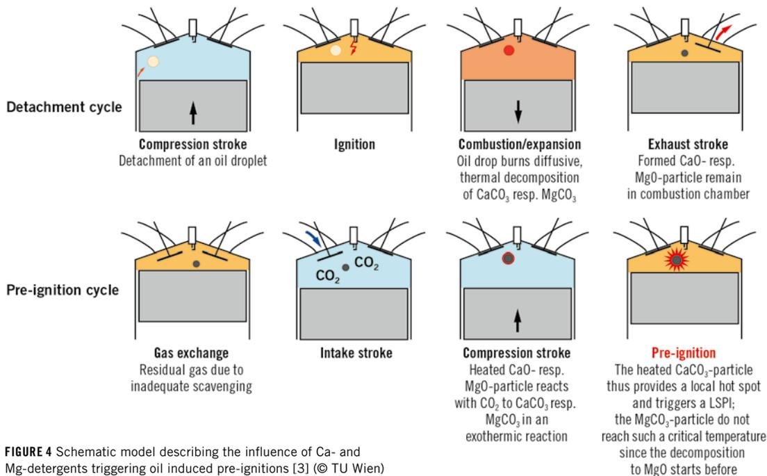
**FIGURE 4** Schematic model describing the influence of Ca- and Mg-detergents triggering oil induced pre-ignitions [3] (© TU Wien)
