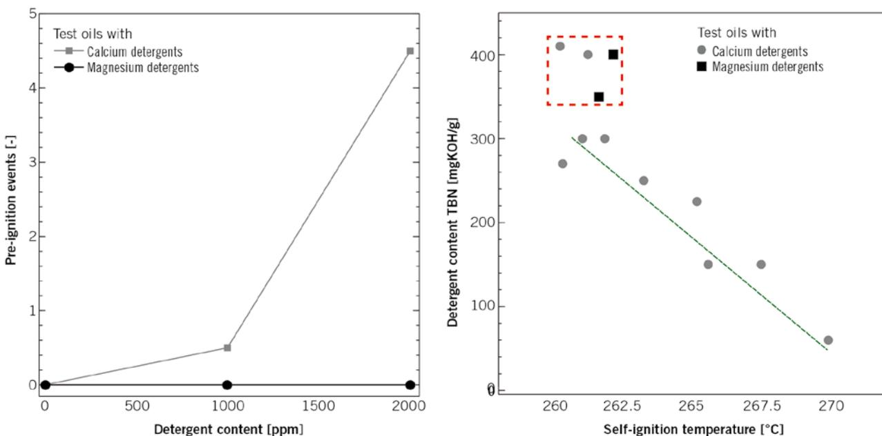
FIGURE 3 Influence of the calcium and magnesium content on the pre-ignition behaviour (left) and influence of metal-based detergents on the self-ignition temperature various test oils according to differential scanning calorimetry at 10 bar (right) (© TU Wien)
