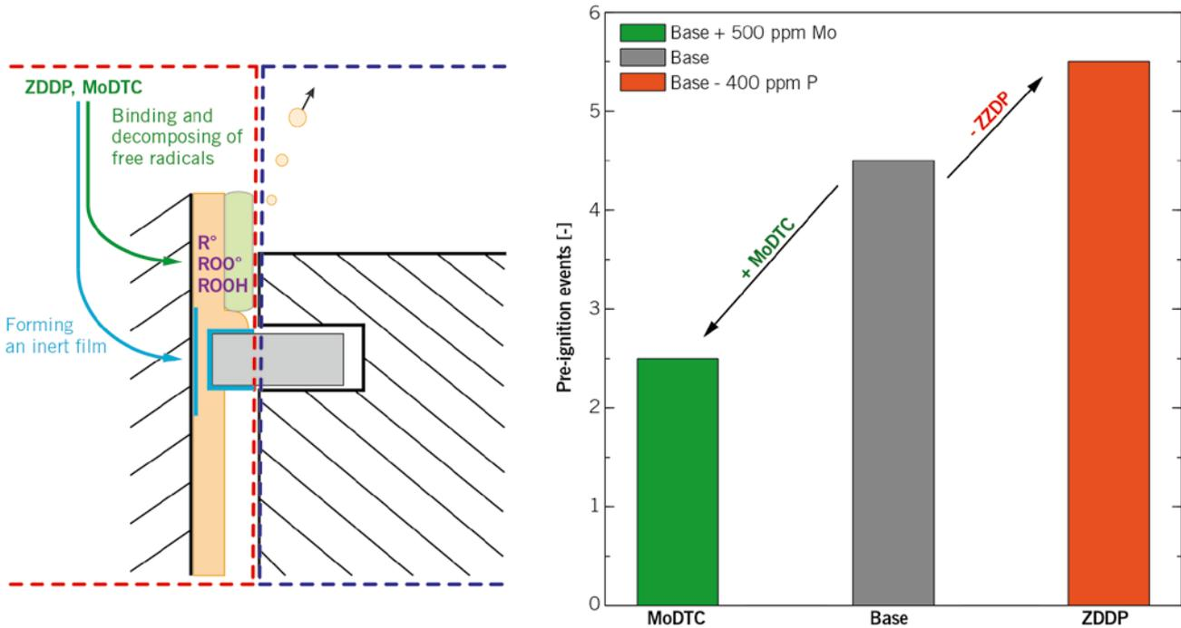
FIGURE 5 Mode of action of antioxidants in the piston crevice volume (left) [3] and influence of various antioxidants on the pre-ignition frequency (right) (© TU Wien)
