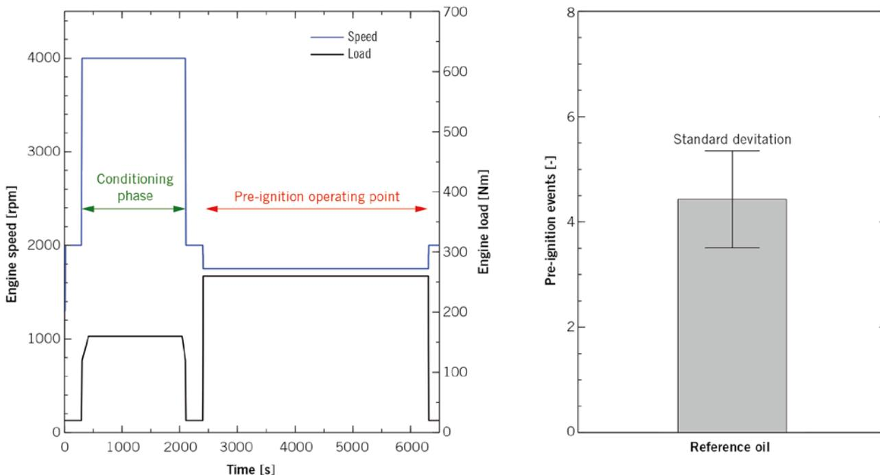
FIGURE 2 Test cycle to verify oil-induced pre-ignitions (left) and illustration of the reproducibility by the reference oil (right) [3] (© TU Wien)
