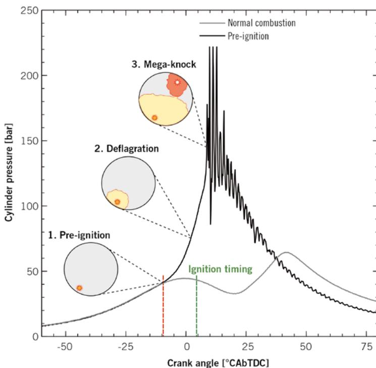
**FIGURE 1** Comparing a pre-ignition with subsequent mega-knock with a cycle of normal combustion [3] (© TU Wien)
